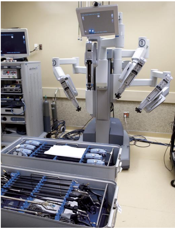
The da Vinci Surgical System enables surgeons to perform an advanced form of laparoscopy.
